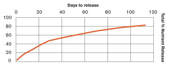
Assessments conducted within controlled 25°C still water. Once 80% of the core has expelled the nutrients, the granule is considered exhausted. Release measurements conducted by the National SCRF Research Centre – Linyi, Shandong Province, China.
